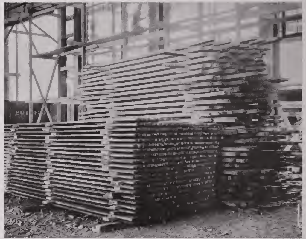
110 TONS OF RAW STEEL FORGING BARS Approximately Million and a Quarter Pounds Received to Date
